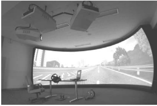
Fig. 10 Three-channel projection system
